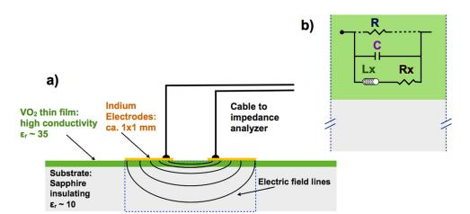
FIG. 1. (a) Measurement setup for inplane impedance spectroscopy of a 90 nm-thick VO<sub>2</sub> thin film at a frequency range 100 Hz-10 MHz between 290 and 345 K. (b) Equivalent circuit of the device. R-C models the insulating contributions to the total impedance, whereas the R<sub>x</sub>L<sub>x</sub> branch models the inductive response from the sample.
