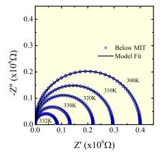
FIG. 2. IS data collected below the MIT, plotted as the negative imaginary vs. real part of the impedance (-Z'' vs. Z'). Open symbols indicate the data; solid (black) lines represent the fit of the data to the model shown in Fig. 1(b).
