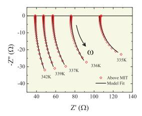
FIG. 3. IS data collected above the MIT, plotted as the negative imaginary vs. real part of the impedance (-Z'' vs. Z'). Open symbols indicate the data; solid (black) lines represent the fit of the data to the model shown in Fig. 1(b).
