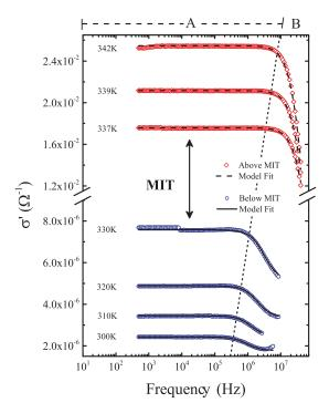
FIG. 4. IS data collected below and above the MIT, plotted as real part of the conductivity  $\sigma'$  vs. f. Open symbols indicate the data, solid and dashed lines represent the fit of the data to the model shown in Fig. 1(b), below and above the MIT, respectively. The data fall into two frequency regimes (regimes A and B) as indicated by the dotted line. The MIT appears as a jump from  $\approx 8 \times 10^{-6} \ \Omega^{-1}$  to  $\approx 1.6 \times 10^{-2} \ \Omega^{-1}$ .
